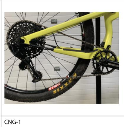
b. Align the chain guide so that it is perpendicular (90 degrees) to the chain.
