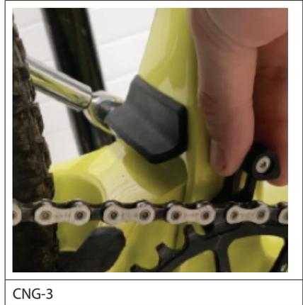
2. Hold the chain guide in place while torquing.
