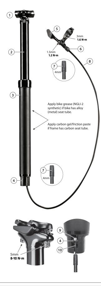
Using a thin coating of friction paste for carbon frames and NGLI-2 synthetic 6. assembly grease for metal frames on the outer tube of the post.
